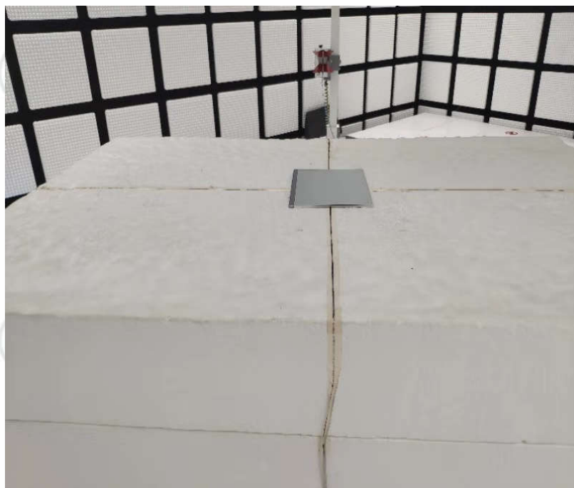
Radiated spurious emission Test Setup-2(Above 1GHz)
