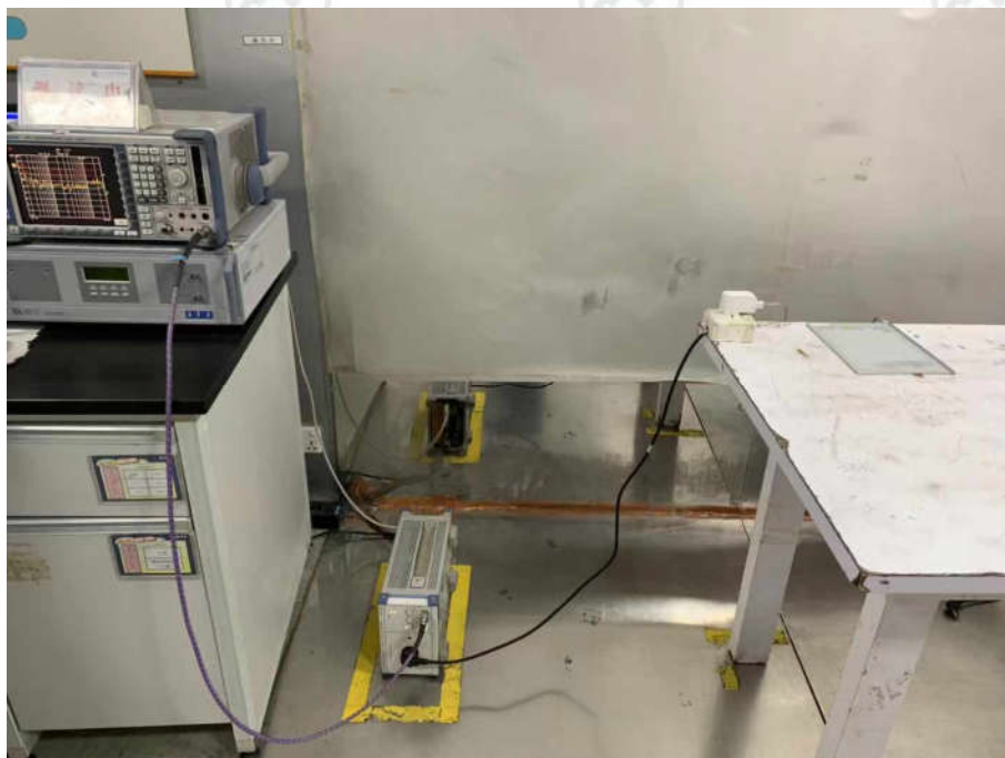
Conducted Emissions Test Setup
