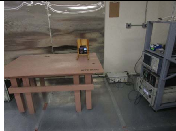
AC Line Conducted Emissions– Front View
