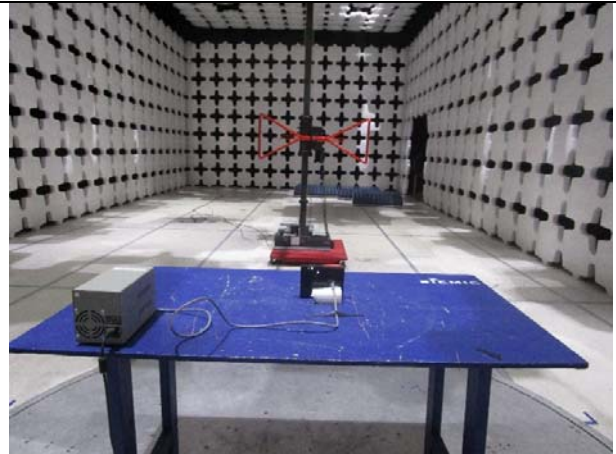
Radiated Emissions (<1GHz) – Rear View
