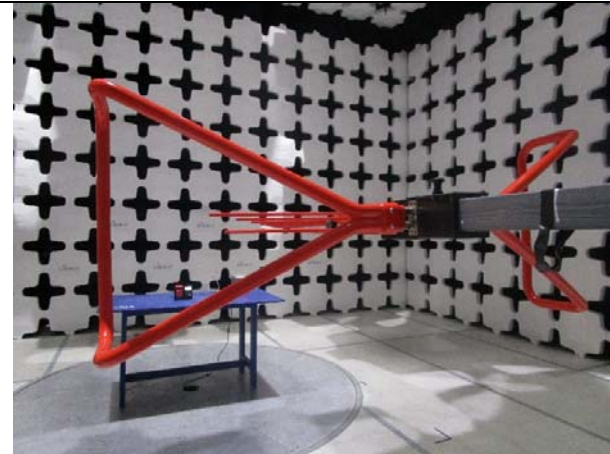
Radiated Emissions (<1GHz) – Front View
