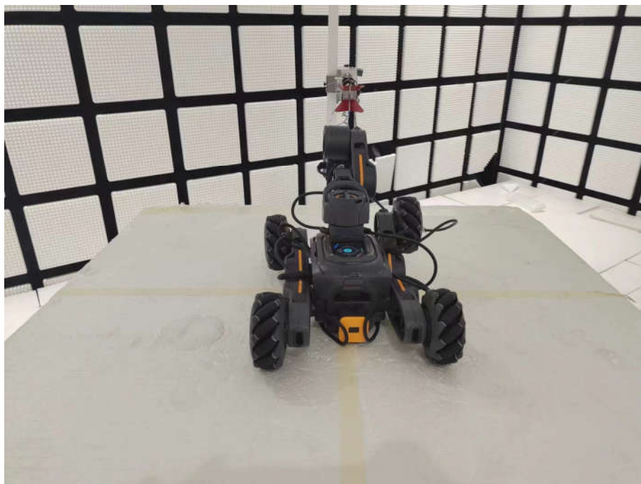
Radiated spurious emission Test Setup-2(Above 1GHz)
