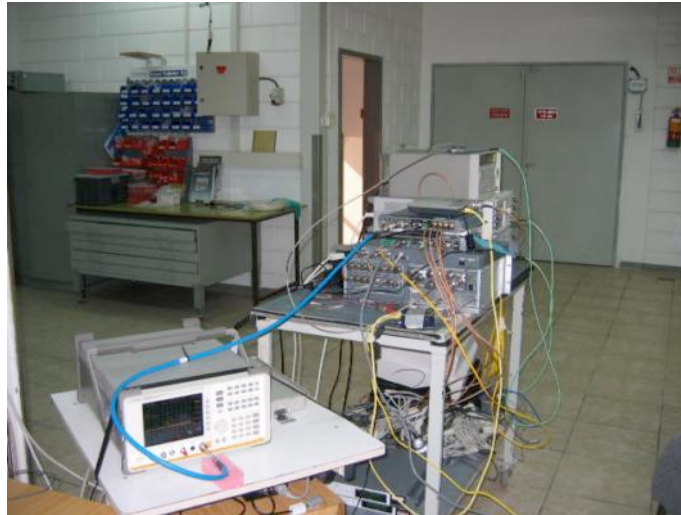
Photograph 1.4.1 Peak output power test setup
