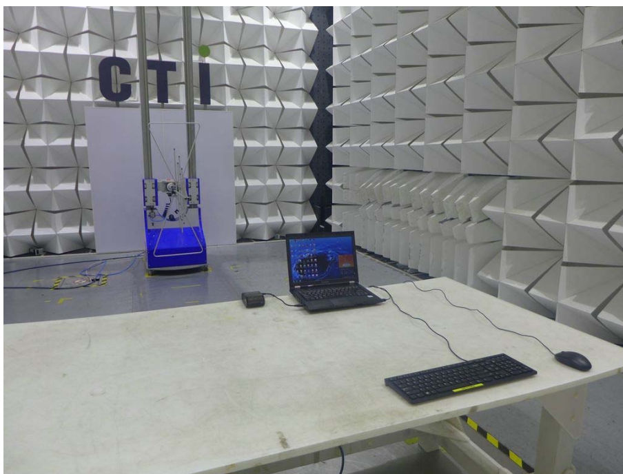
Radiated emission Test Setup-2 (30MHz-1GHz)
