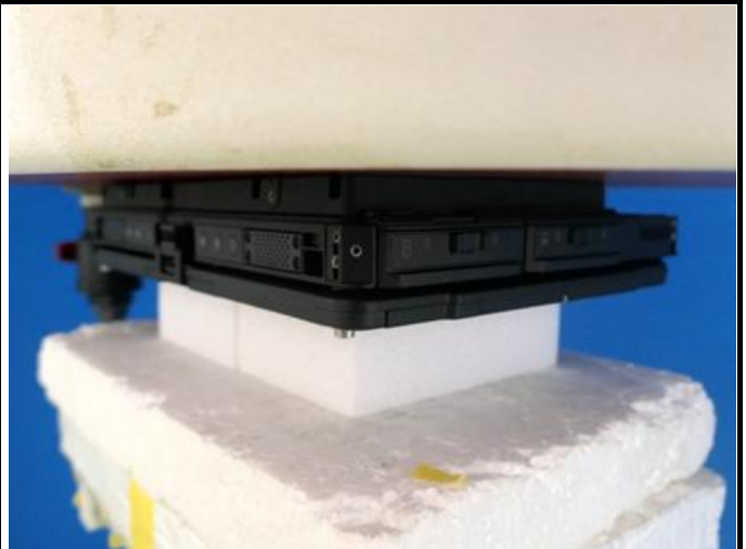
Rear Face of EUT with 0 mm Gap
