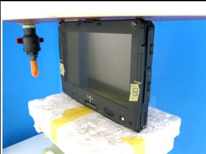
Top Side of EUT with 0 mm Gap
