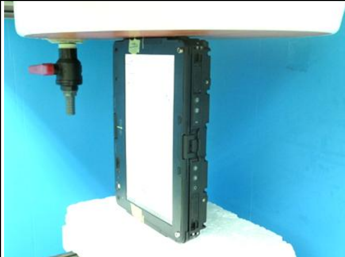
Left Side of EUT with 0 mm Gap
