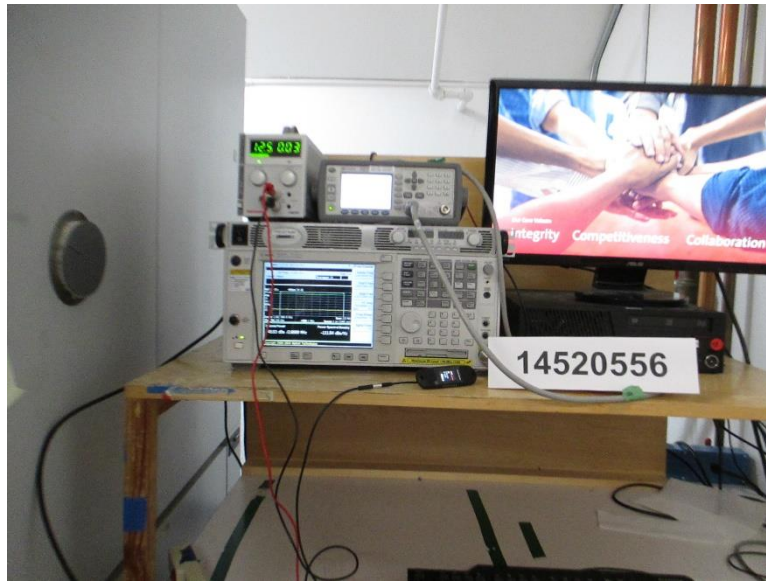
RF ANTENNA PORT CONDUCTED
