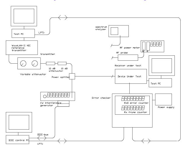
Figure 1, measurement test set-up.
