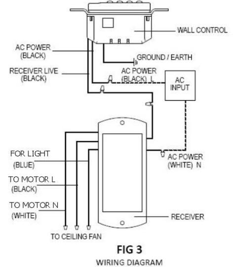
AC POWER ON/OFF SWITCH (
