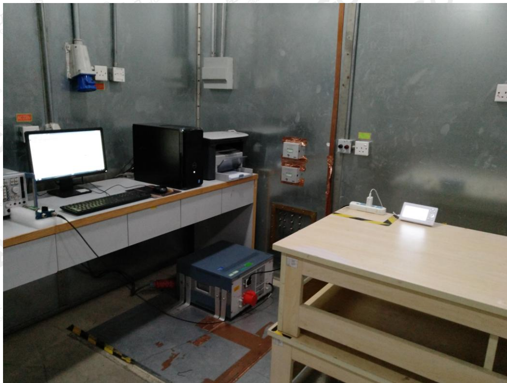
RADIATED EMISSION TEST SETUP BELOW 1GHZ
