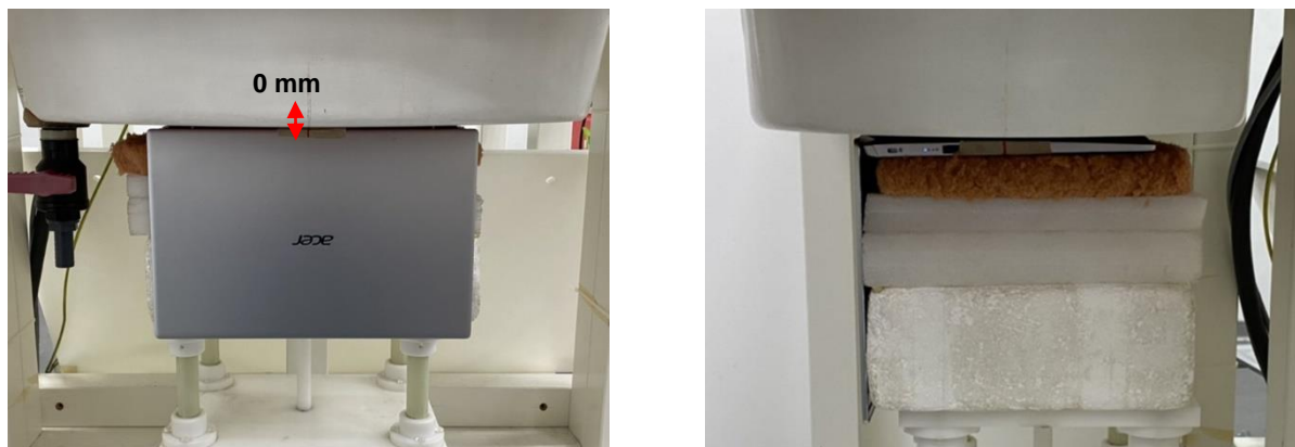
Fig.3 EUT Bottom side to flat phantom
