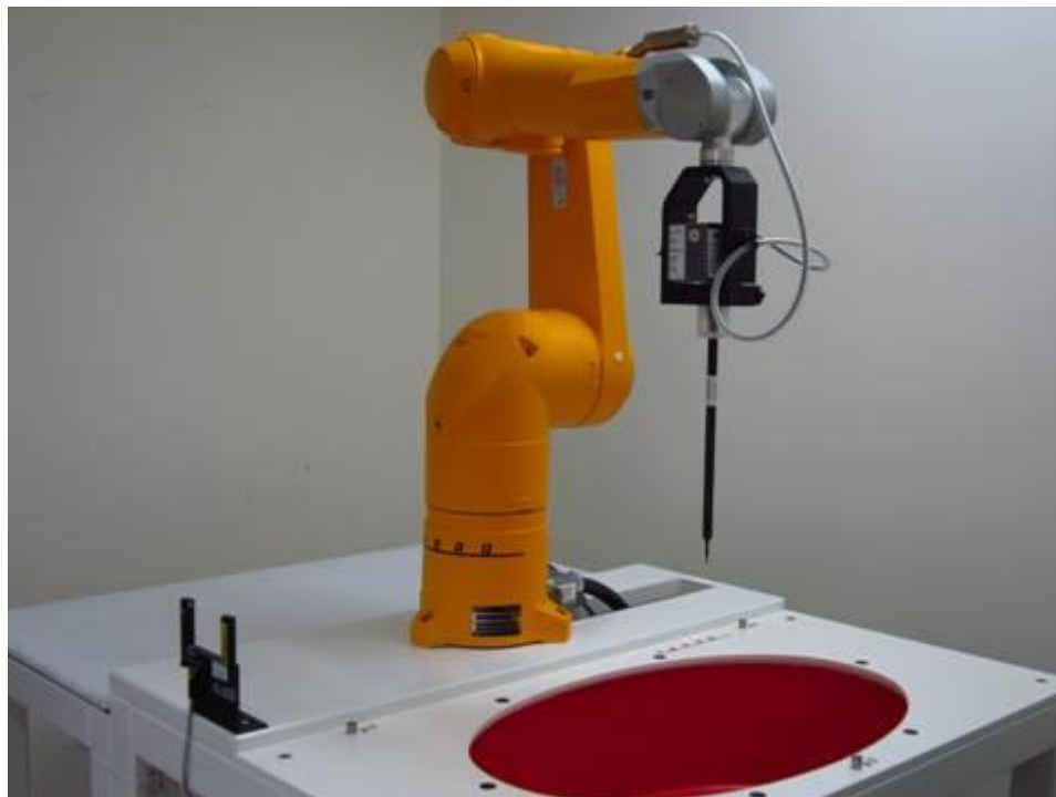
Fig.1 Photograph of the SAR measurement system
