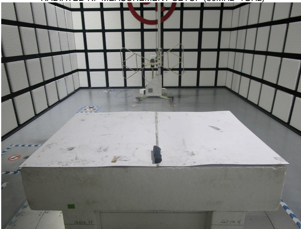
RADIATED RF MEASUREMENT SETUP (30MHz~1GHz)
