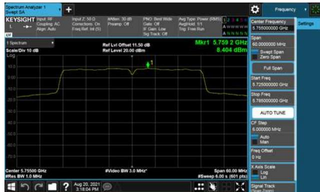
Modulation Type: 802.11ac VHT80 (29.3Mbps)
