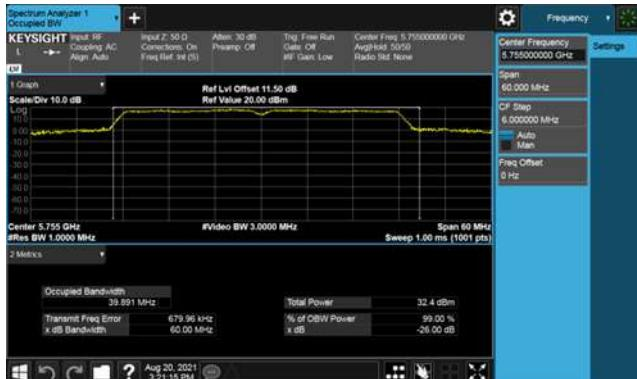
Modulation Type: 802.11ac, VHT80 (29.3Mbps)
