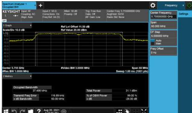
Modulation Type: 802.11ac, VHT80 (29.3Mbps)
