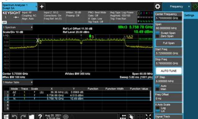
Modulation Type: 802.11ac, VHT80 (29.3Mbps)
