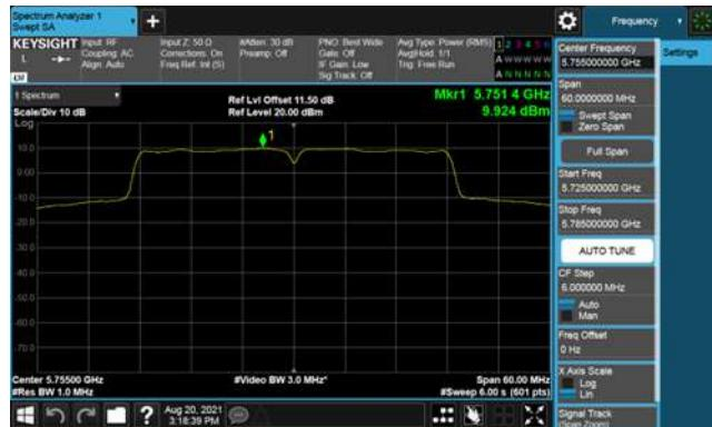
Modulation Type: 802.11ac VHT80 (29.3Mbps)
