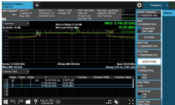
Modulation Type: 802.11ac, VHT20 (6.5Mbps)
