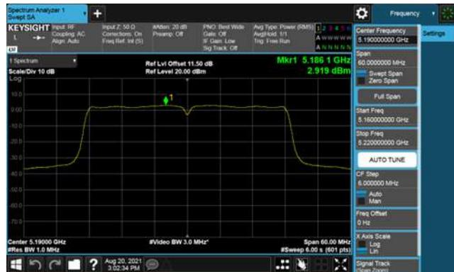
Modulation Type: 802.11ac VHT80 (29.3Mbps)
