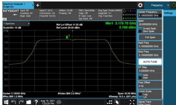
Modulation Type: 802.11ac VHT20 (6.5Mbps)
