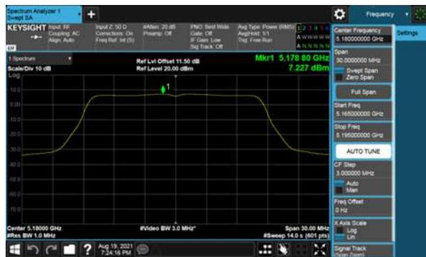
Modulation Type: 802.11ac VHT20 (6.5Mbps)
