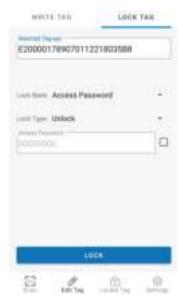
Touch to choose the lock band and the lock type from the drop-down list. Enter the access password if necessary and touch **LOCK**.
