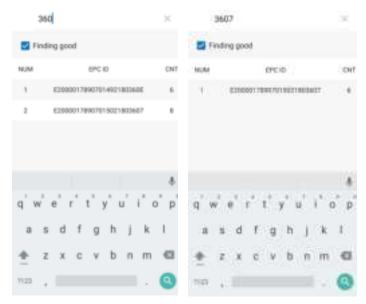
3. Select the tag you want and check "Finding good". Touch Scan to go back to the Scan screen. The located tag is highlighted in the list.
