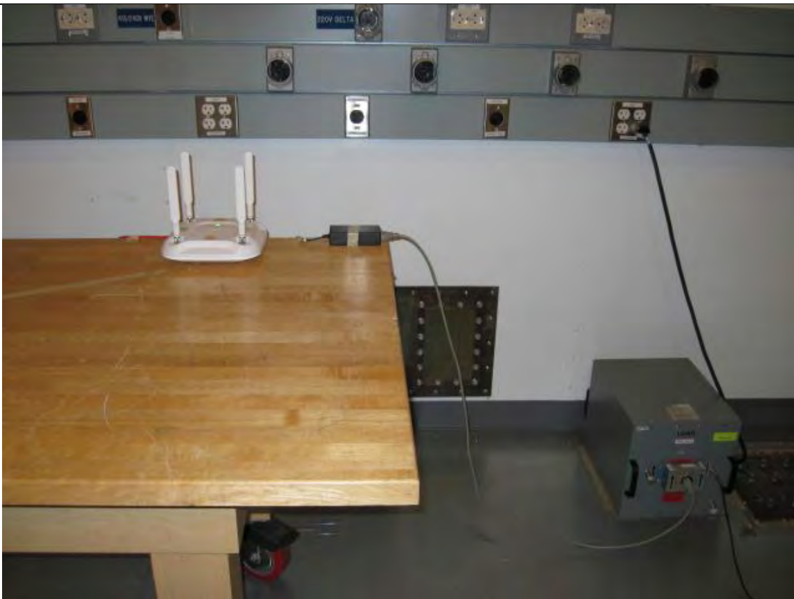
Title: Power Line Conducted Emissions Test Setup
