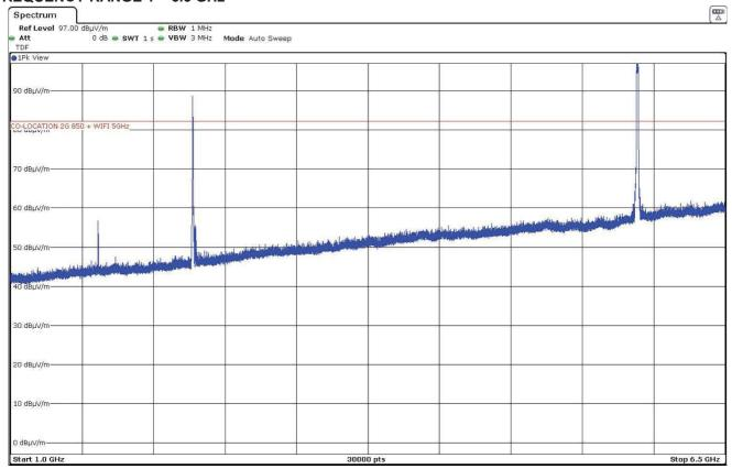
The peak above the limit on the left is the Carrier frequency Bluetooth Low Energy (2402 MHz). The peak above the limit on the right is the Carrier frequency 802.11 a20 U-NII-3 (5825 MHz).
