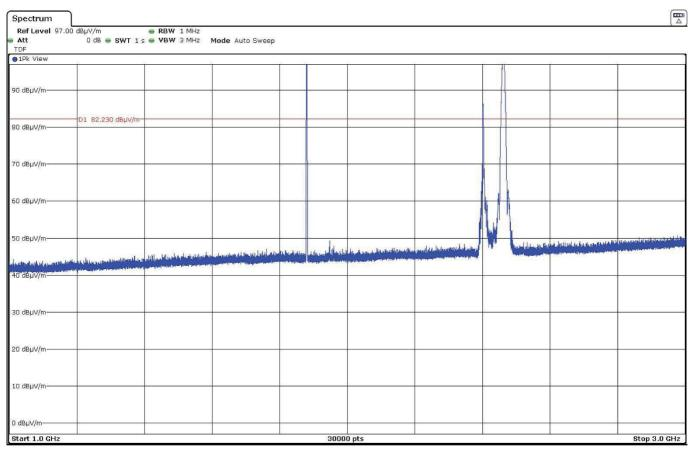
The peak above the limit on the left is the Carrier frequency 2G Band PCS-1900 (1909.8 MHz).
