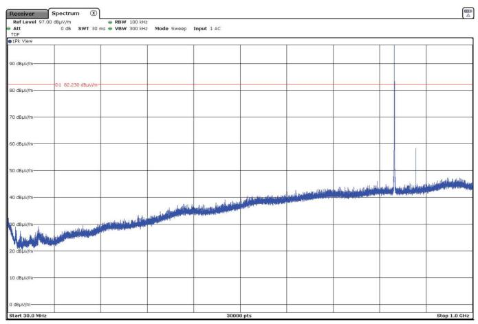
The peak above the limit is the Carrier frequency 2G Band GSM-850 (836.6 MHz). The other peak at 881.6 MHz corresponds to the downlink signal 2G Band GSM-850.
