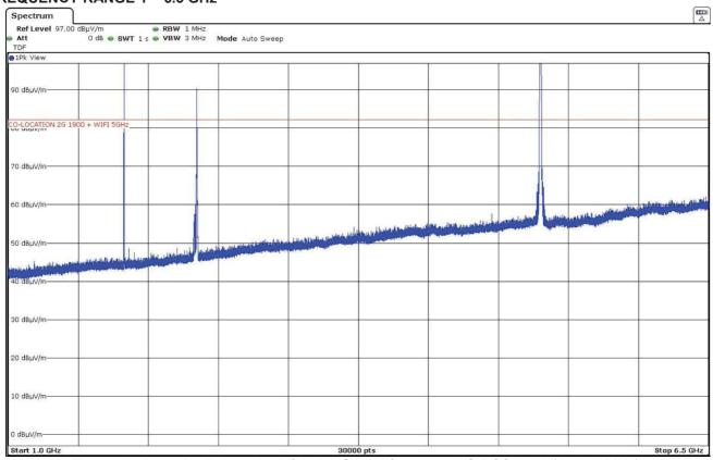
The peak above the limit on the left is the Carrier frequency 2G PCS-1900 (1909.8 MHz). The peak above the limit in the middle is the Carrier frequency Bluetooth Low Energy (2480 MHz). The peak above the limit on the right is the Carrier frequency 802.11 a20 (5180 MHz).
