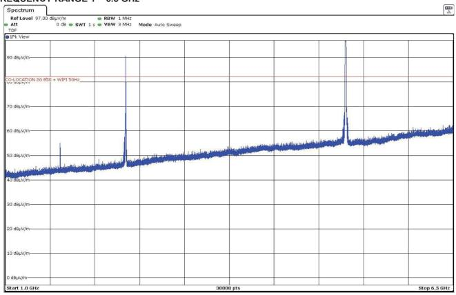
The peak above the limit on the left is the Carrier frequency Bluetooth Low Energy (2480 MHz).
