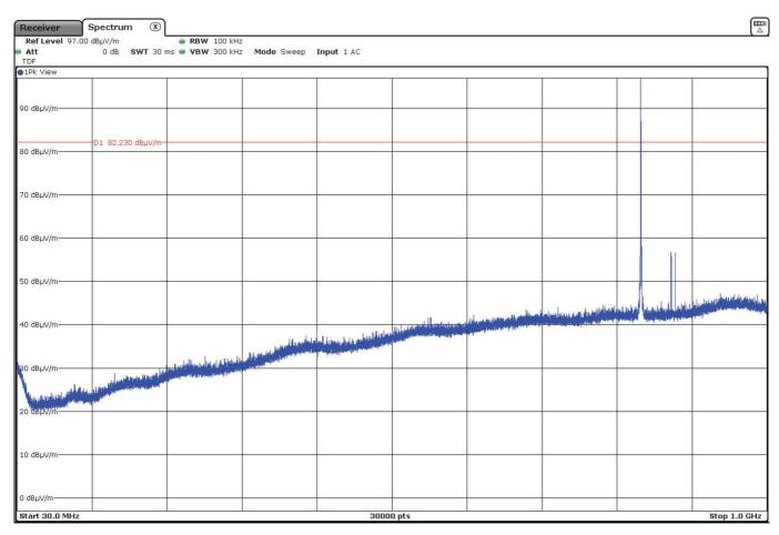
The peak above the limit is the Carrier frequency 2G Band GSM-850 (836.6 MHz). The peak at 881.6 MHz corresponds to the downlink signal 2G Band GSM-850.
