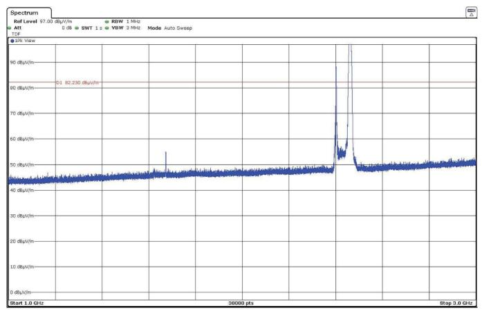
The peak above the limit on the left is the Carrier frequency Bluetooth Low Energy (2402 MHz).
