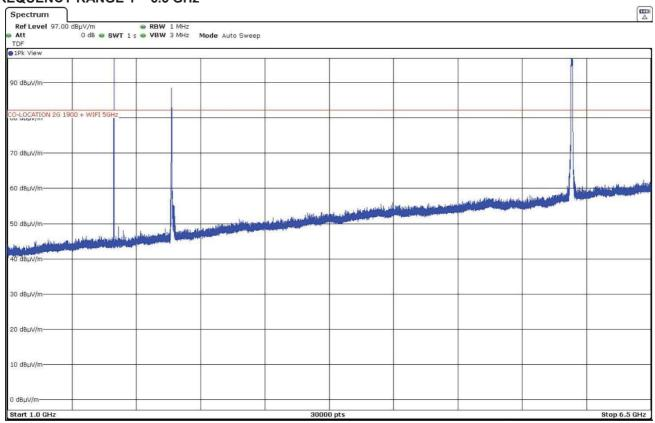
The peak above the limit on the left is the Carrier frequency 2G PCS-1900 (1909.8 MHz). The peak above the limit in the middle is the Carrier frequency Bluetooth Low Energy (2402 MHz) The peak above the limit on the right is the Carrier frequency 802.11 a20 (5825 MHz).
