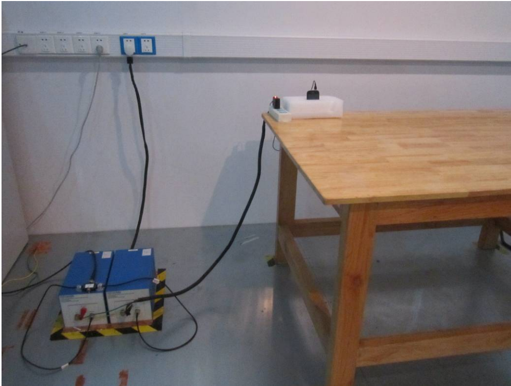
Conducted Emissions Test Setup Front View
