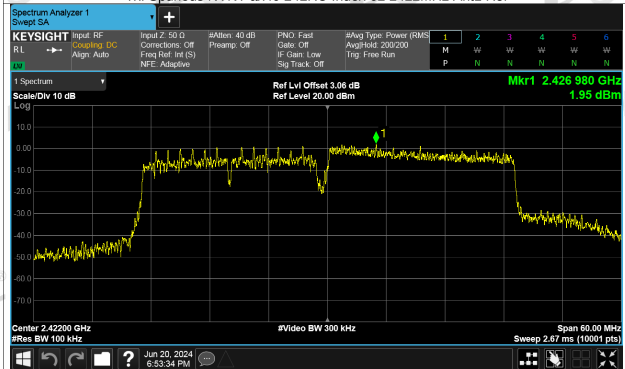
Tx. Spurious NVNT ax40 242RU Index 62 2422MHz Ant1 Emission
