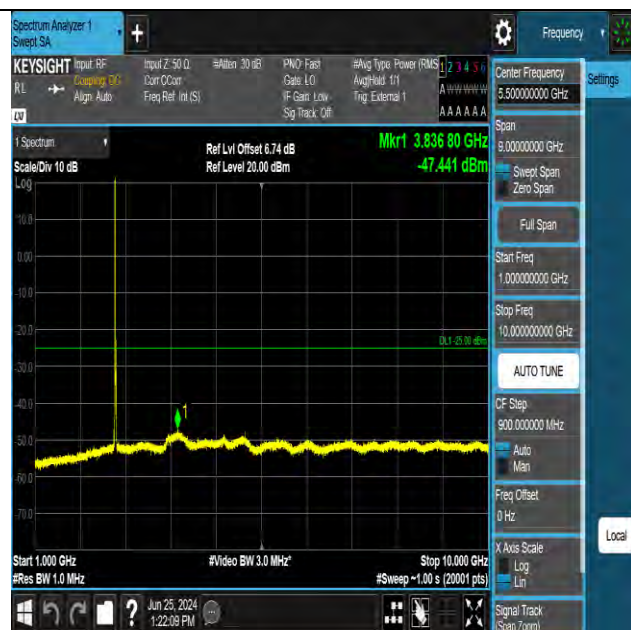
Band41 15MHz QPSK 40620 1RB#0 1000~10000 1000~10000
