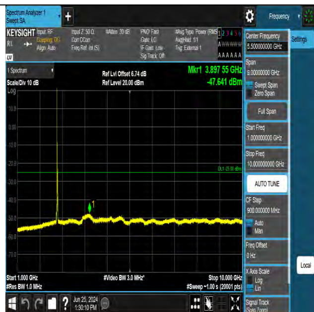
Band41 20MHz QPSK 40620 1RB#0 1000~10000 1000~10000
