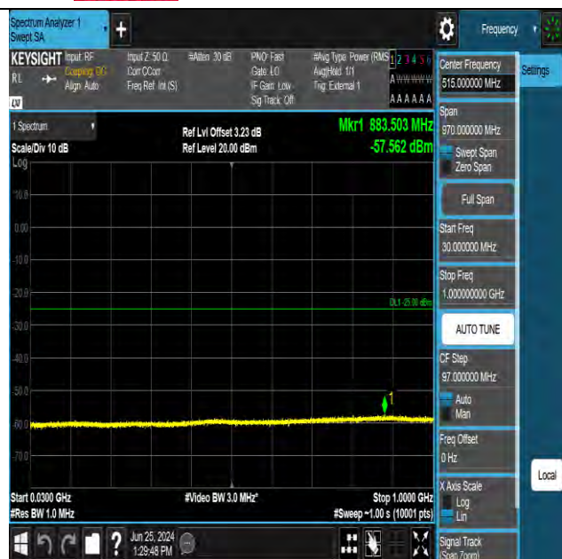
Band41 20MHz QPSK 40620 1RB#0 30~1000 30~1000
