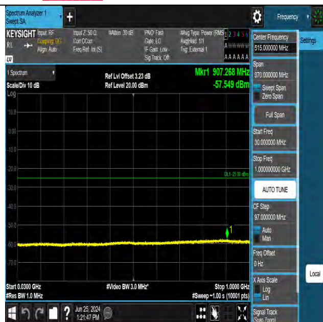
Band41 15MHz QPSK 40620 1RB#0 30~1000 30~1000
