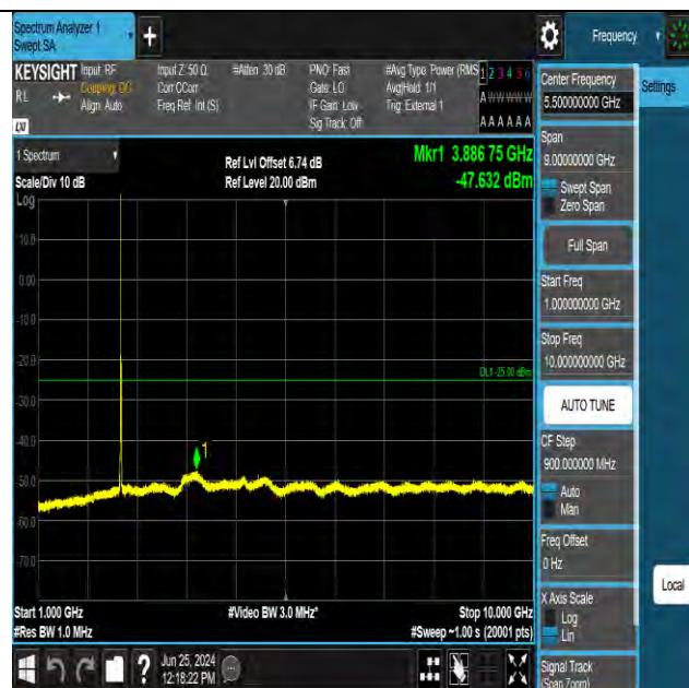
Band41 10MHz QPSK 39700 1RB#0 1000~10000 1000~10000
