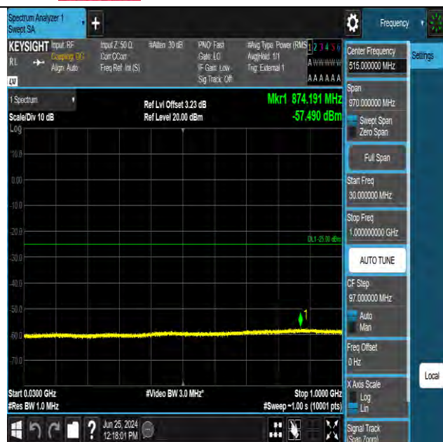
Band41 10MHz QPSK 39700 1RB#0 30~1000 30~1000
