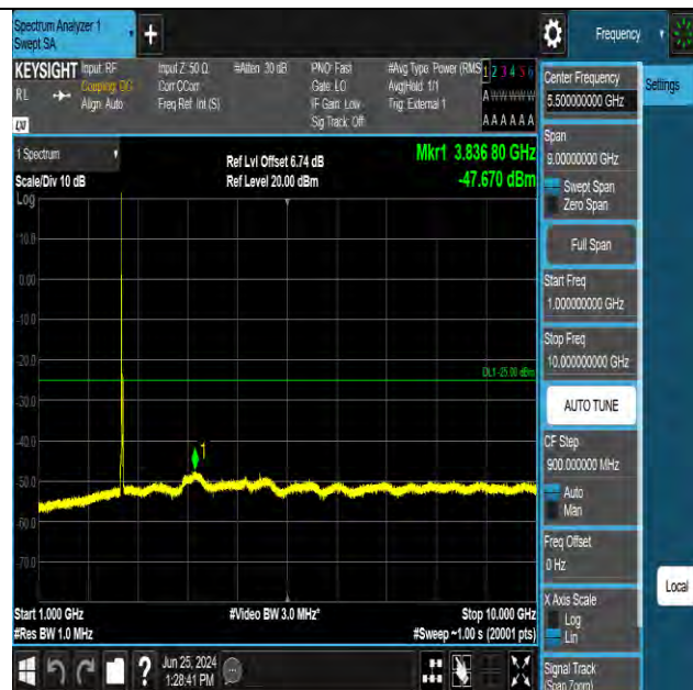
Band41 20MHz QPSK 39750 1RB#0 1000~10000 1000~10000
