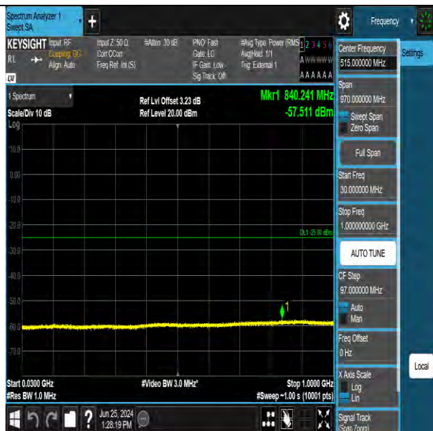
Band41 20MHz QPSK 39750 1RB#0 30~1000 30~1000
