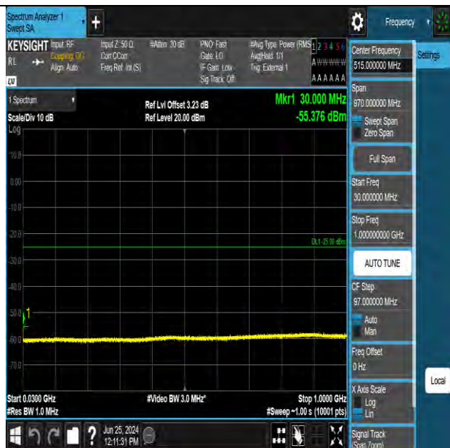
Band41 5MHz QPSK 40620 1RB#0 30~1000 30~1000
