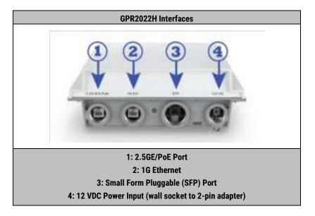
Interfaces are recessed at the bottom of the unit.
