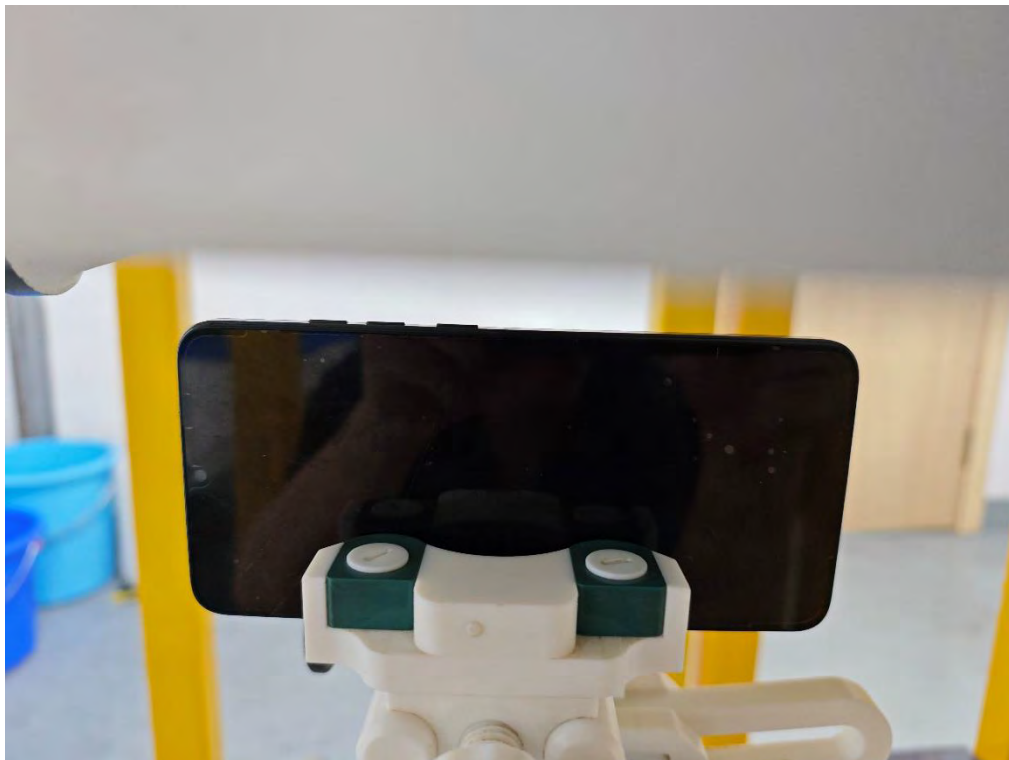
Body Edge 2(Right) (separation distance is 10mm)
