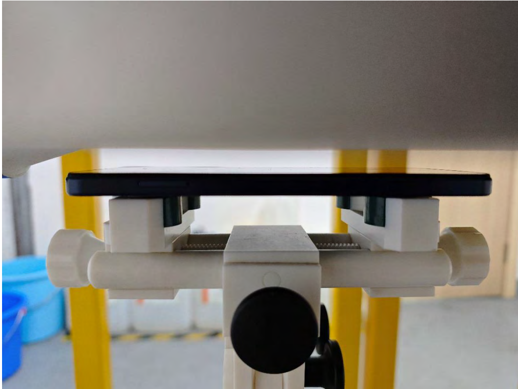
Body Back side(separation distance is 10mm)
