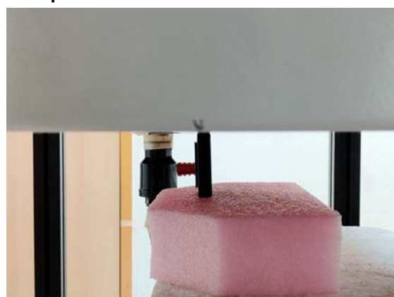
Fig.5 EUT Bottom side to flat phantom
