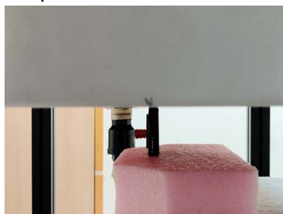
Fig.4 EUT Top side to flat phantom
