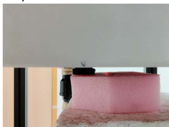
Fig.8 EUT Front side to flat phantom
