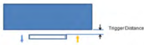
Picture : Proximity Sensor Triggering Distances Assessment(Back/Front Side)
