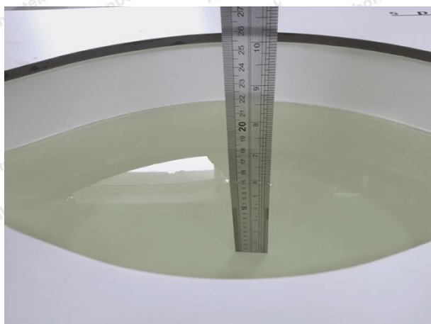
Liquid depth in the body phantom (2450MHz)
