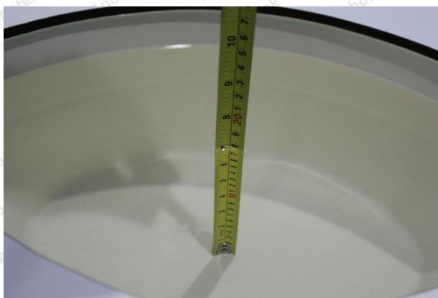
Liquid depth in the body phantom (5GHz)
