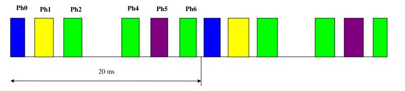
Ph0: **Emitting**. The microprocessor make the oscillator and the amplifier on.
