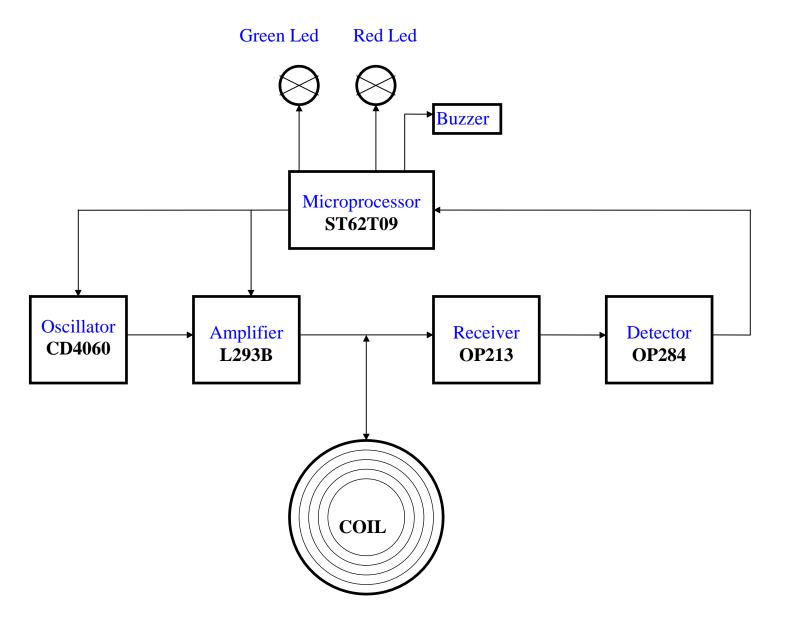
The oscillator generate a tension of which frequency is about 58 kHz.
