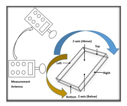
Note: The measurement antenna are moving and surrounding the EUT when performed the test, the test results recorded the highest values for each sides of the EUT (left/right/top/bottom/z-axis)
