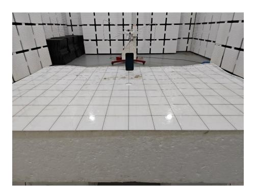
Set-up for Radiated Spurious Emission, Above 1GHz
