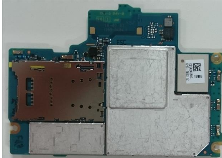
Internal PWB with Shield cases (Front-side)
