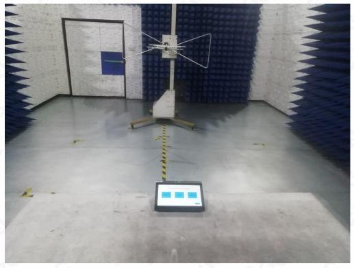
FCC RADIATED EMISSION TEST SETUP ABOVE 1GHZ
