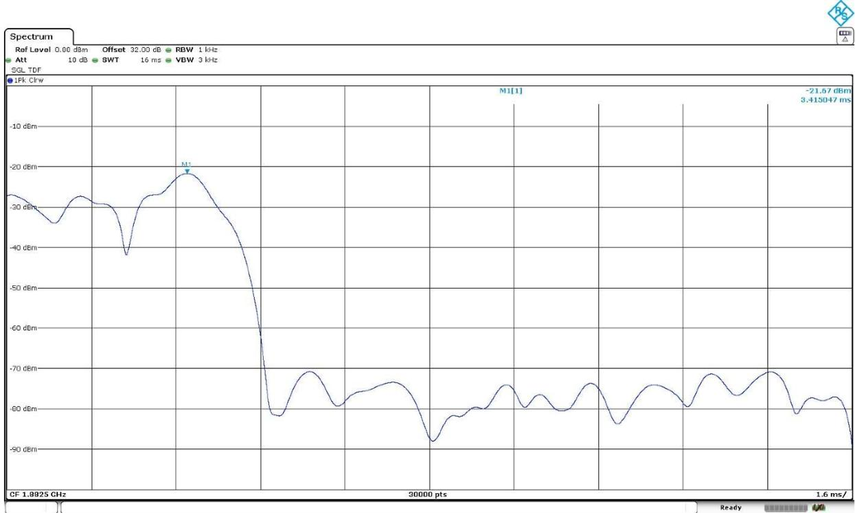
**LTE Cat NB1 Band 25: Pi/4-QPSK. Middle Channel. BW=3.75 kHz. Tone Number=1. Tone Offset=0. MSC/TBS=3.**
