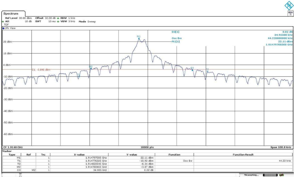
LTE Cat NB1 Band 25. Pi/4-QPSK. BW=3.75 kHz. Tone Number=1. Tone Offset=23. MSC/TBS=3.
