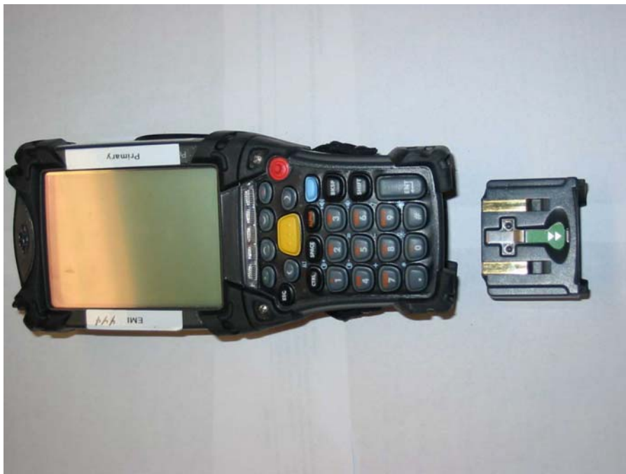
Figure 4 – MC9063 with Battery Removed
