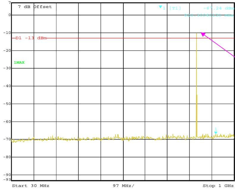
Fundamental test with notch filter
