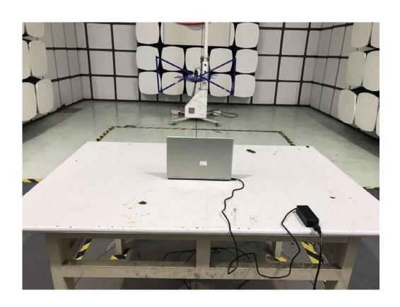
**Radiated Test (Above 1GHz)**
