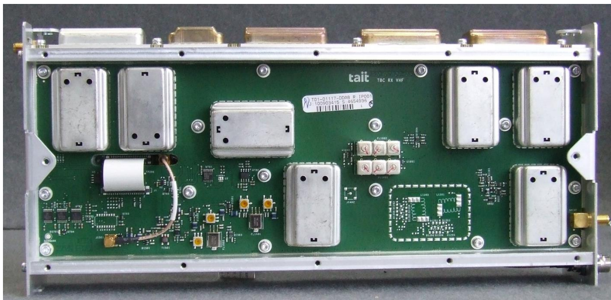
Photograph 17: Receiver Board (RXB) – Top
