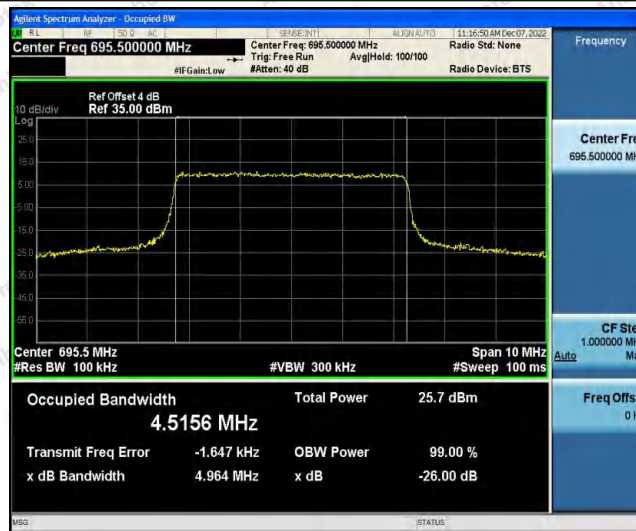
Band71-5MHz-16QAM-133147-25RB#0
