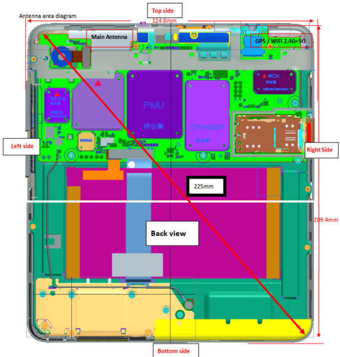
Picture 11.1 Antenna Locations (Back View)
