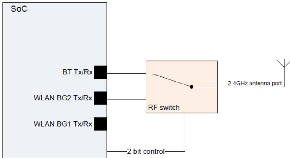
Figure 4. Wi-Fi – BT/BLE Coexistence – Shared Antenna
