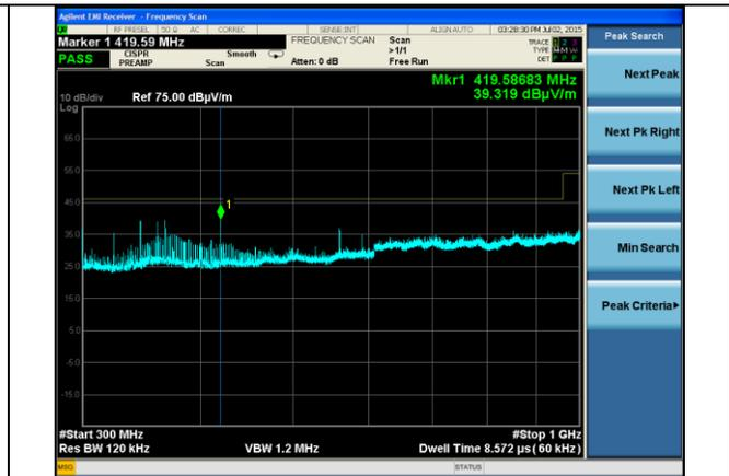
Horizontal Transmitter enabled
