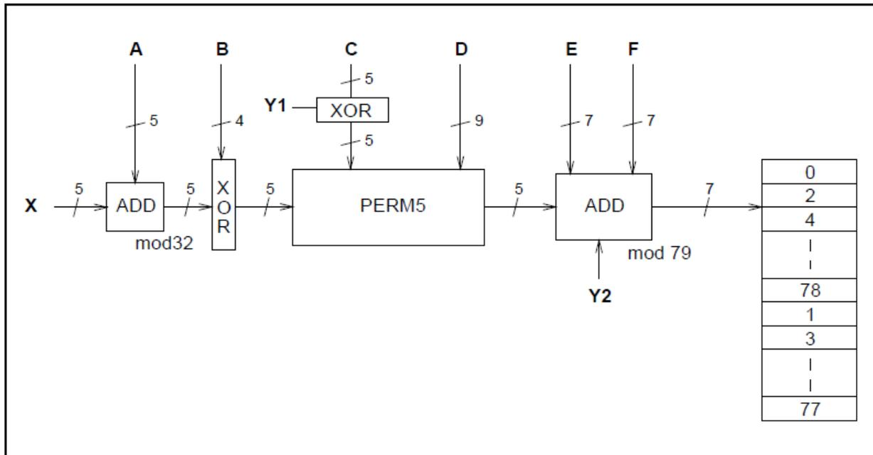
The X input determines the phase in the 32-hop segment, whereas Y1 and Y2 selects between master-to-slave and slave-to-master. The inputs A to D determine the ordering within the segment, the inputs E
