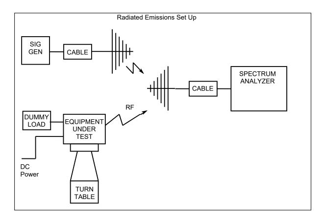
All other testing is performed using the **T**eltest **R**adio **EVA**luation system (TREVA), which is configured as shown below. The Spectrum Analyser is connected to the EUT via the attenuator network for Conducted Emissions testing, and Occupied Bandwidth.
