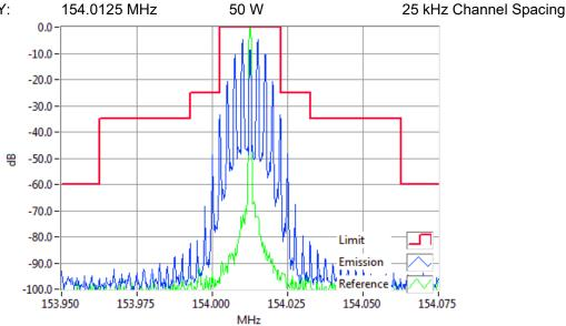
Analogue Modulation 154.0125MHz Mask B 50W RBW=300Hz, VBW=3000Hz, Detector Mode=Peak Result=Pass
