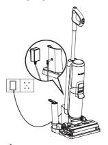
To charge the appliance, place the appliance on the charging dock and plug the adaptor into a power outlet.
