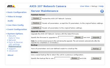
**Notes:** •After starting the upgrade process, always wait at least 10-15 minutes before restarting the camera, even if you suspect the upgrade has failed.
