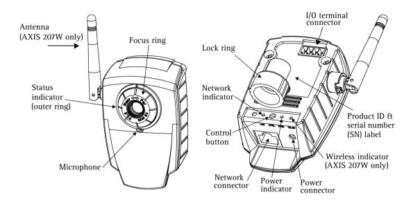
**Antenna (AXIS 207W only)** - For connection to wireless networks. Compatible with IEEE802.11g networks at speeds of up to 54 Mbit/s.
