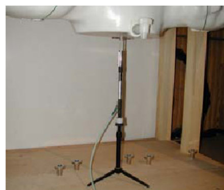
Figure 12.1 Dipole Validation Test Setup
