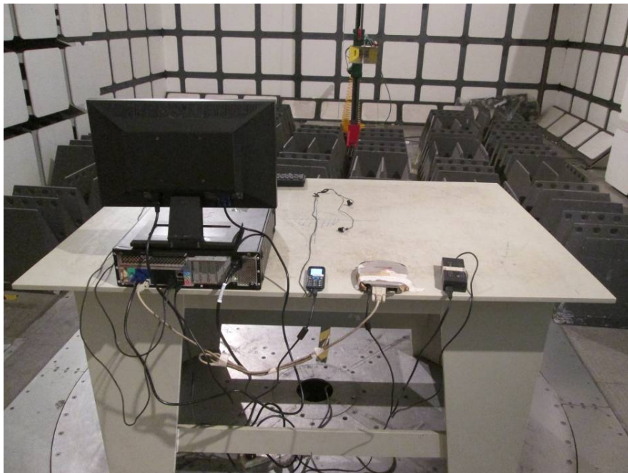
Radiated Emissions – Rear View (Above 1 GHz)
