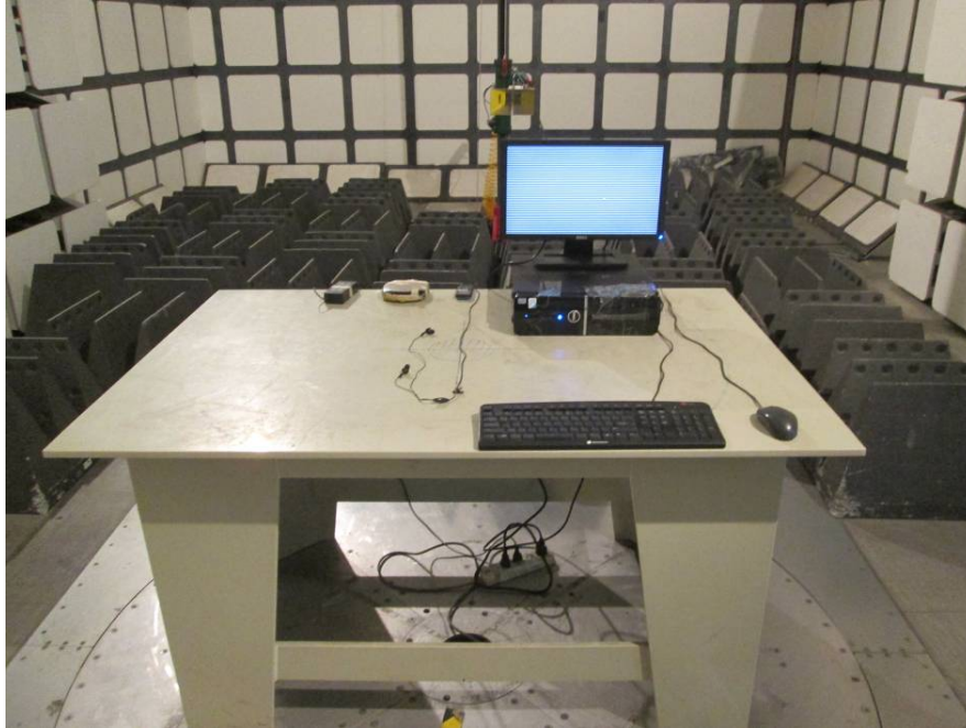
Radiated Emissions – Front View (Above 1 GHz)
