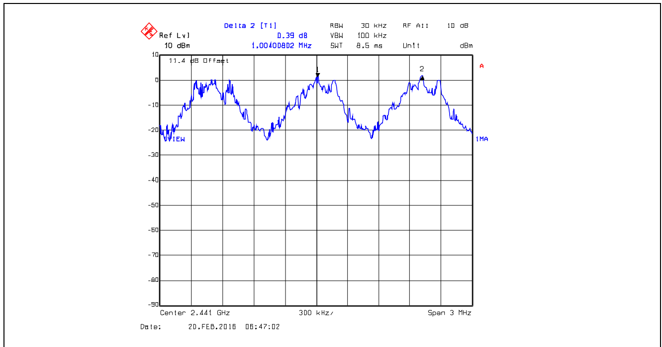
Plot 5.3.4.2.1. Carrier Frequency Separation, GFSK, DH1, CH 39, 2441 MHz
