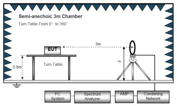
(B) Radiated Emission Test-Up Frequency 30MHz~1GHz
