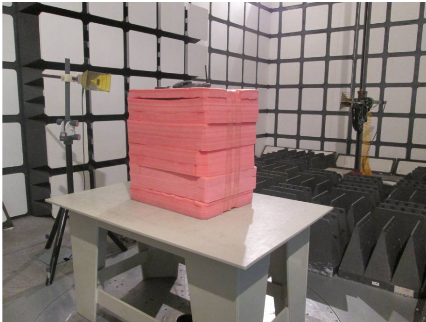
Radiated Emissions Test View (Above 1 GHz)
