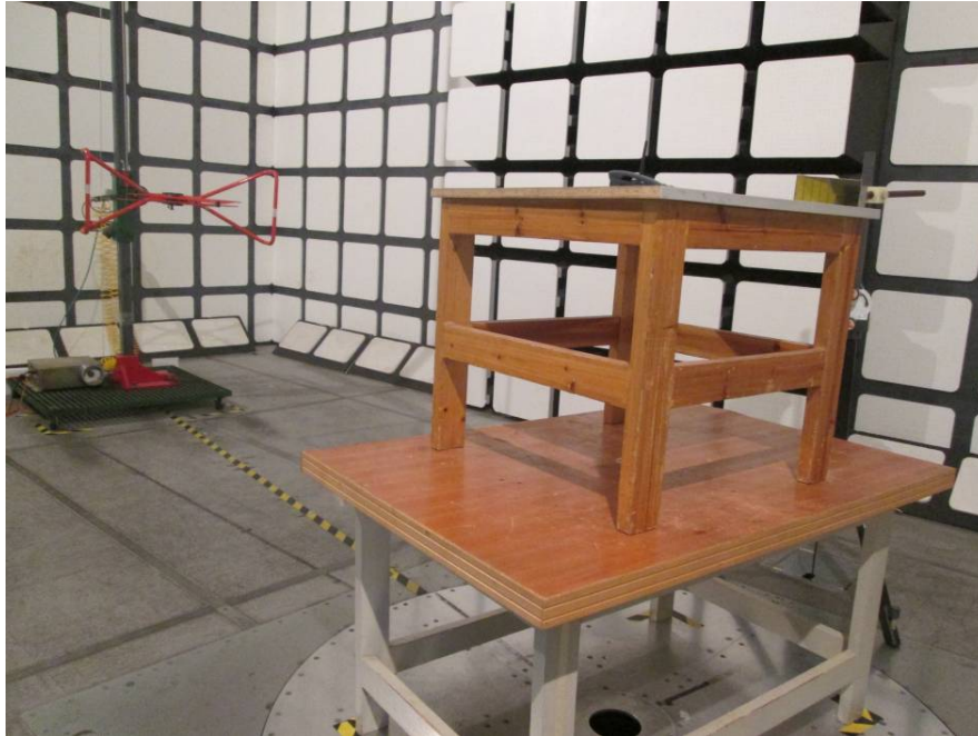
Radiated Emissions Test View (Below 1 GHz)
