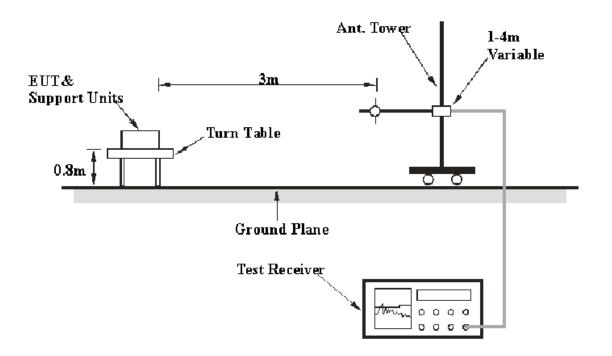
The radiated emission tests were performed in the open area 3-meter test site, using the setup accordance with the FCC MP - 5. The specification used was the FCC part 18 Subpart C limits.
