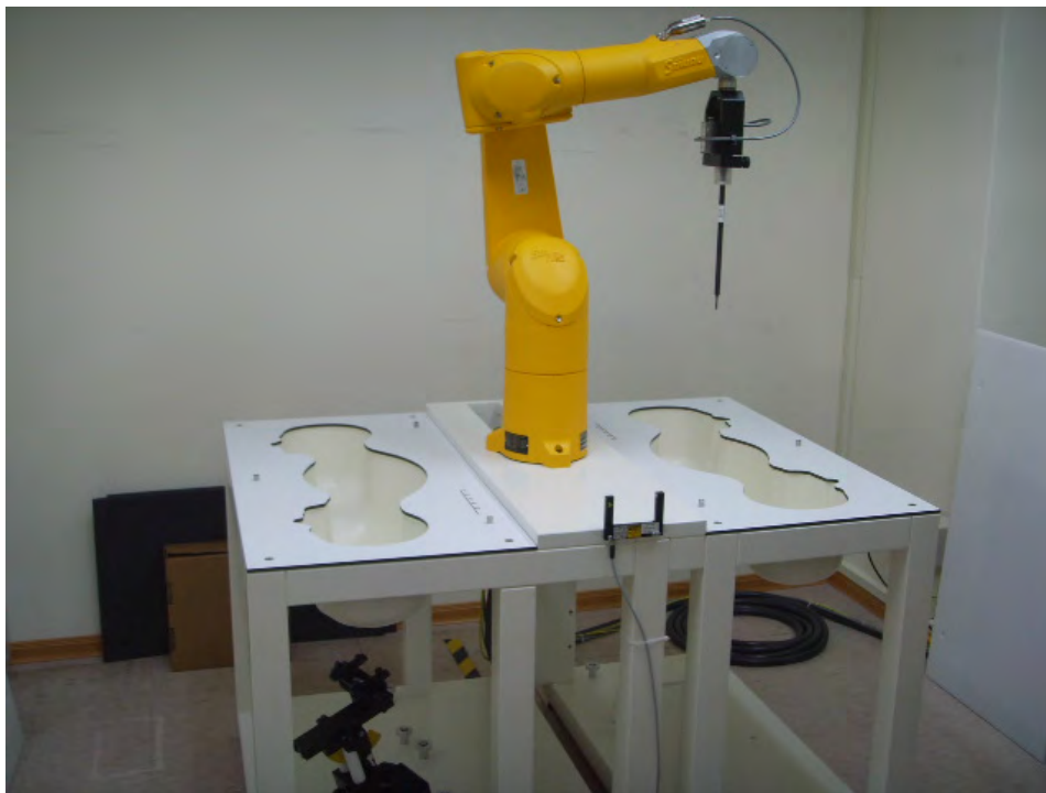
Fig.1 Photograph of the SAR measurement system
