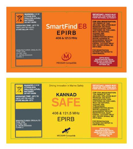
The beacon upper body label is shown in the following image and is the same for all variants. It contains the following information required by C/S T.001 section 3.5.8:
