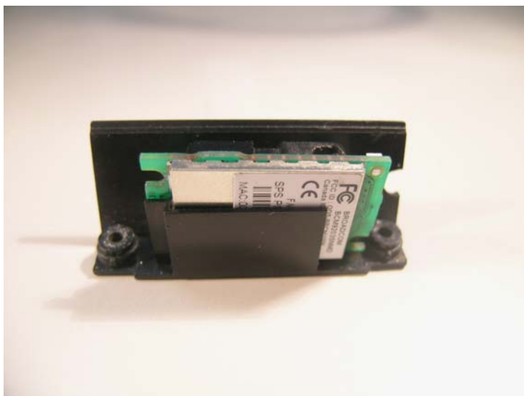
Antenna Module mounted in plastic Holder
