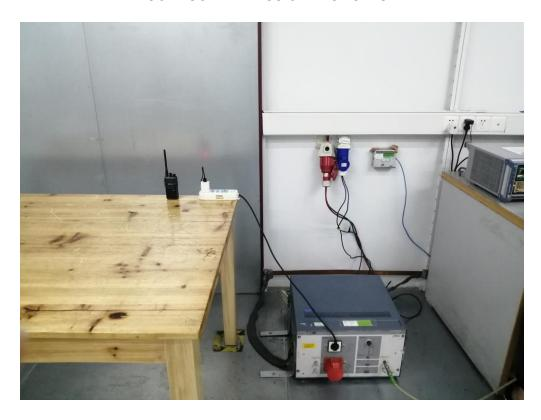
RADIATED EMISSION TEST SETUP-BELOW 1GHZ
